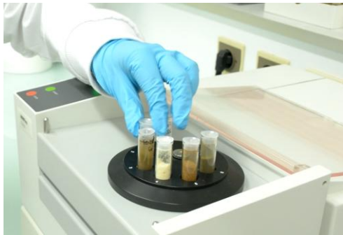
NIRS used for the analysis (Nirflex BÜCHI) Reflectance mode (4000 – 10000 cm -1 )
