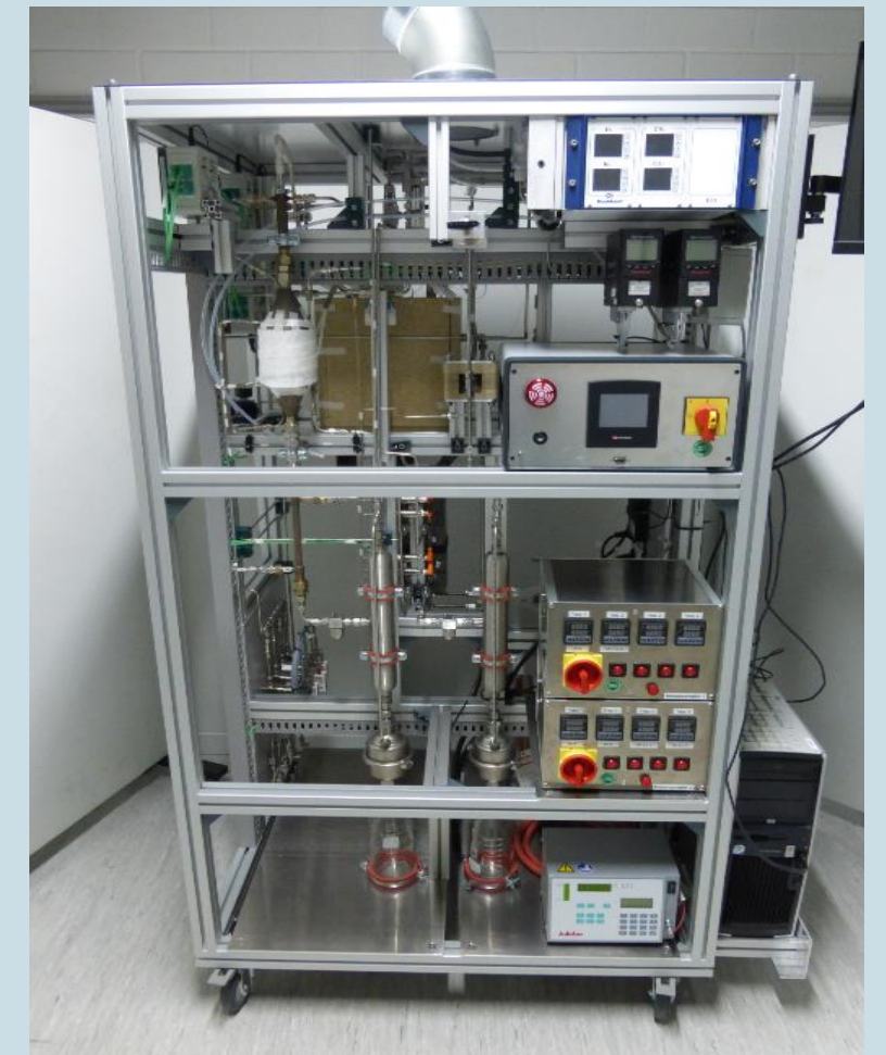
Foto: Mini CO 2 -methanation plant at IMM in Mainz
