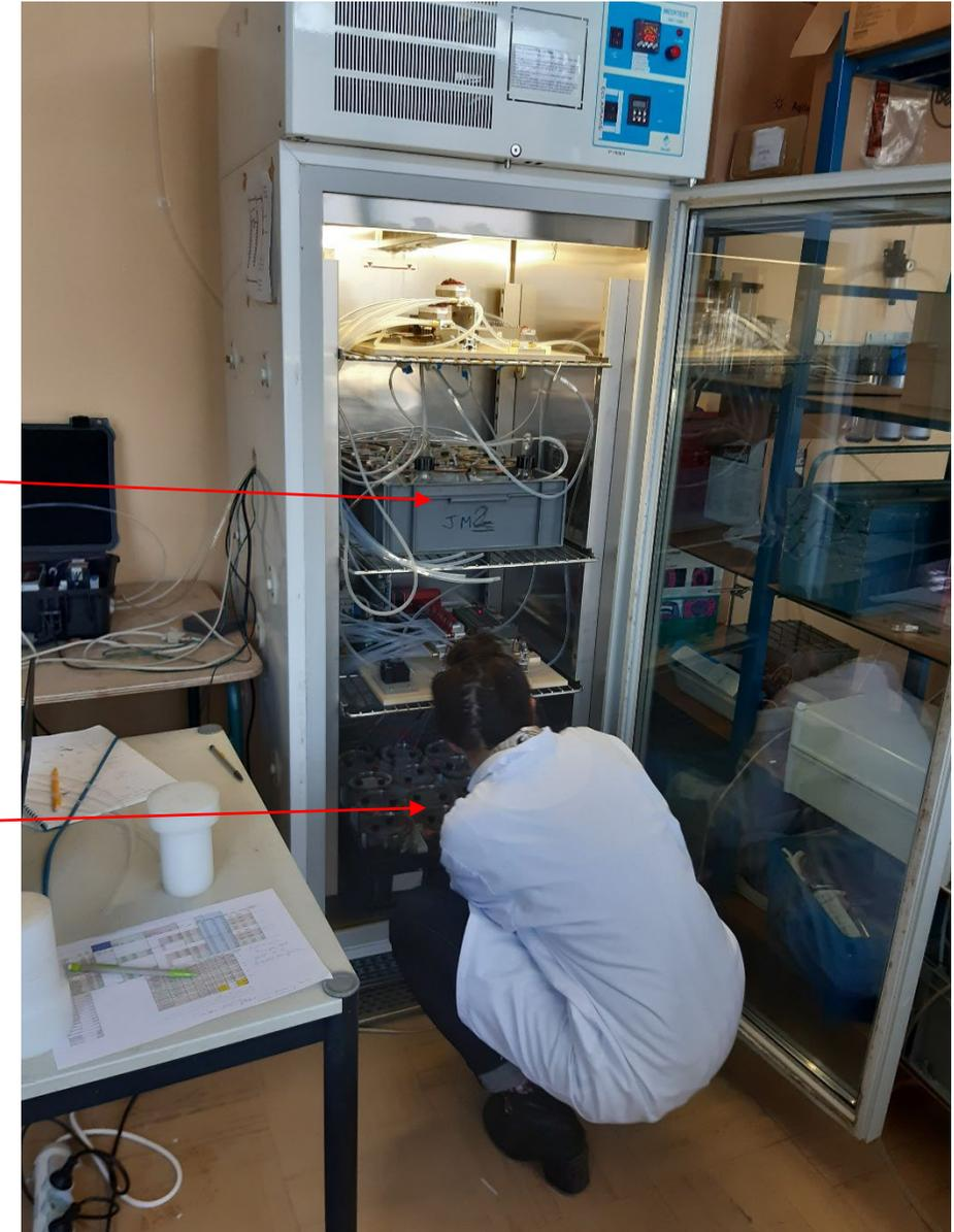
QCL Aerodyne N<sub>2</sub>O, H<sub>2</sub>O, CH<sub>4</sub>
