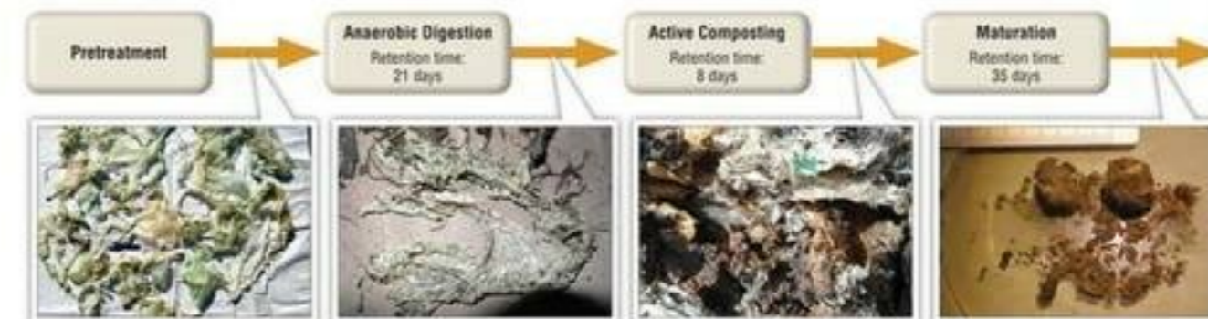
Figure 1. Sampling process and degradation steps in facility 3, Lingen. (Photo on left: washed compostable plastic bag fragments)
