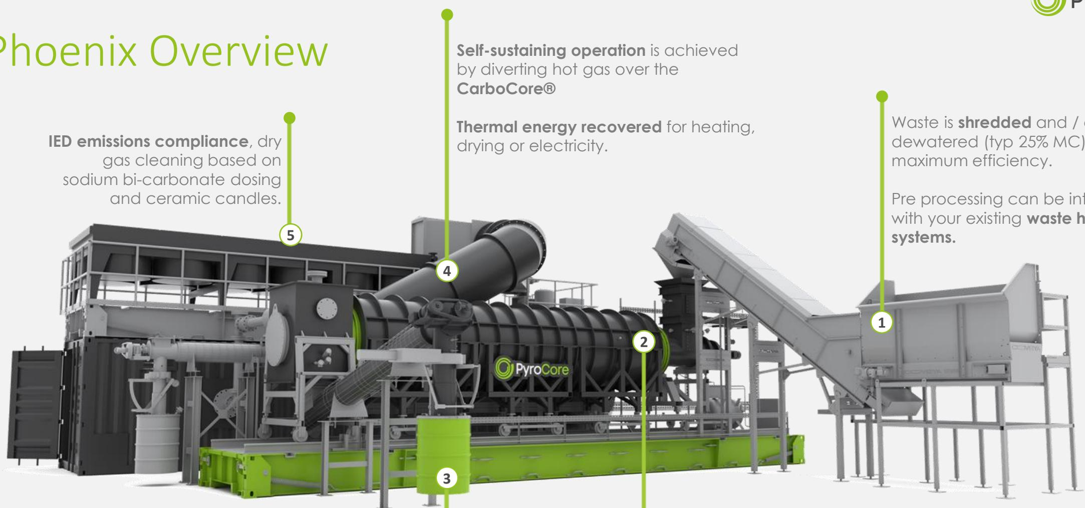
**IED emissions compliance**, dry gas cleaning based on sodium bi-carbonate dosing and ceramic candles.
