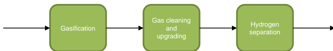
Figure 17: General process layout for hydrogen production via gasification.
