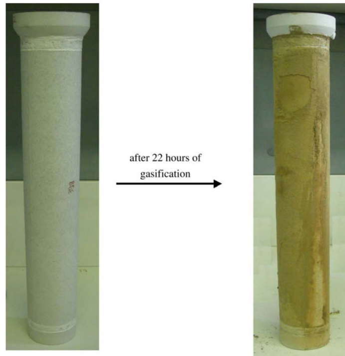
Figure 31: Catalytic ceramic candle before and after the gasification test. (Rapagnà et al., 2010)
