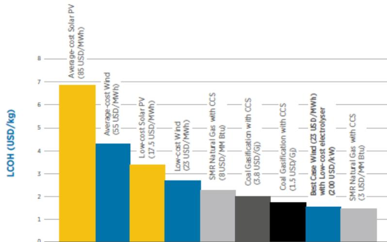
Notes: Electrolyser capex: USD 840/kW; Efficiency: 65%; Electrolyser load factor equals to either solar or wind reference capacity factors. For sake of simplicity, all reference capacity factors are set at 48% for wind farms and 26% for solar PV systems.
